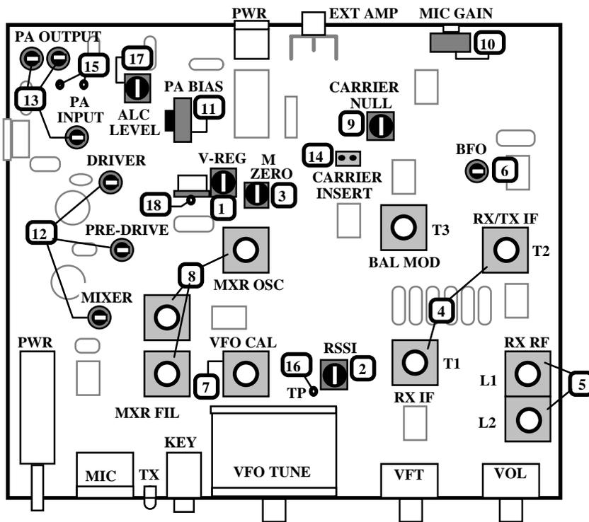
**Note:** For trimpots, trimcaps, and IF cans (T1-T3), use a non-conductive tuning wand with a metallic tip. For TOKO brand inductors, use a non-conductive wand with a narrow plastic tip. For Coilcraft brand inductors, use a small hex-head non-metallic tuning tool.
